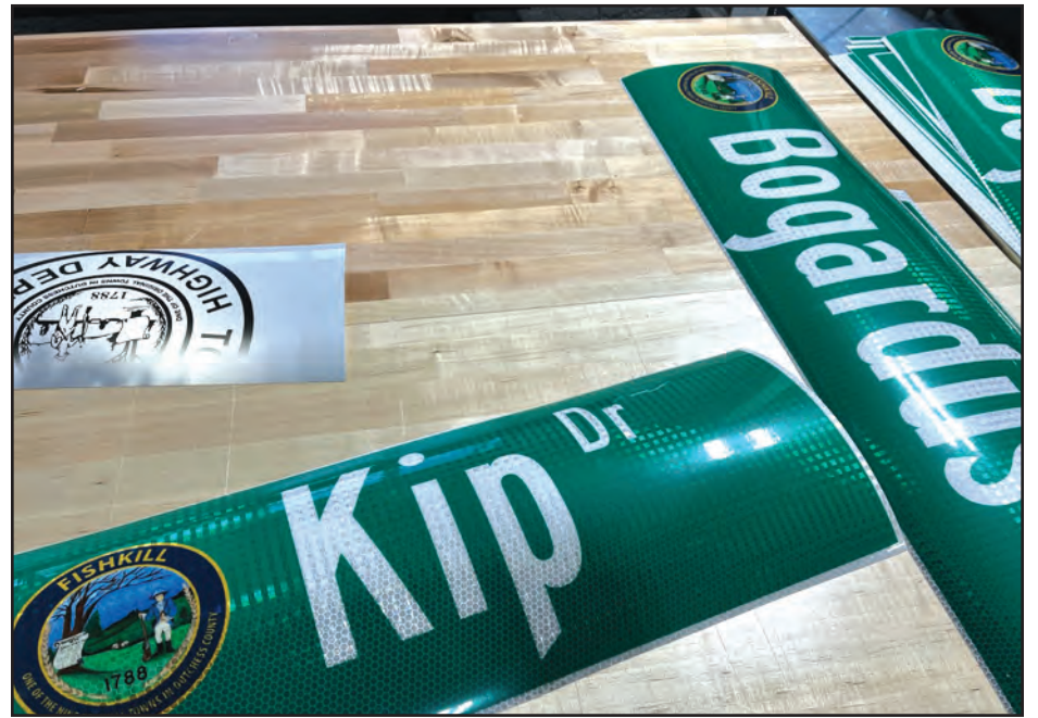
Some of the printed street signs before they are laminated and placed on metal backings.
