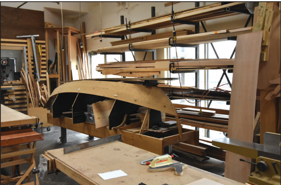
Surrounded by racks of materials, a small lapstrake style flat bottomed dinghy takes shape in the workshop at the Hudson River Wooden Boat School. This project began with an earlier YouthBoat program that had to be put on hold due to COVID. The team at the school are preparing to complete the project with help from the next class of students. Photo by Jim Donick
