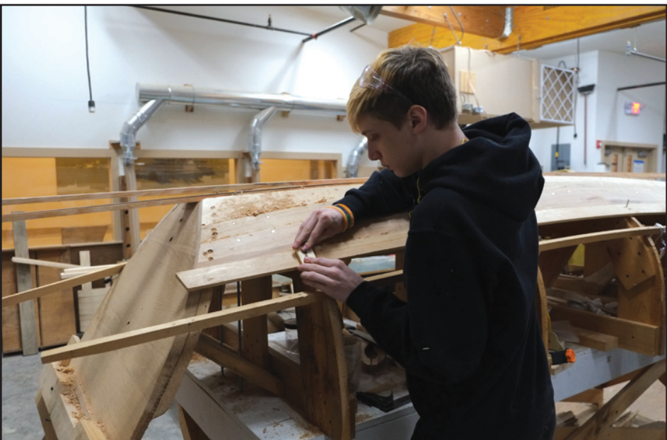
A student in the last pre-COVID class measuring a cedar plank for the hull of the ten foot sailing dinghy that the team constructed. Photo by Jim Donick
