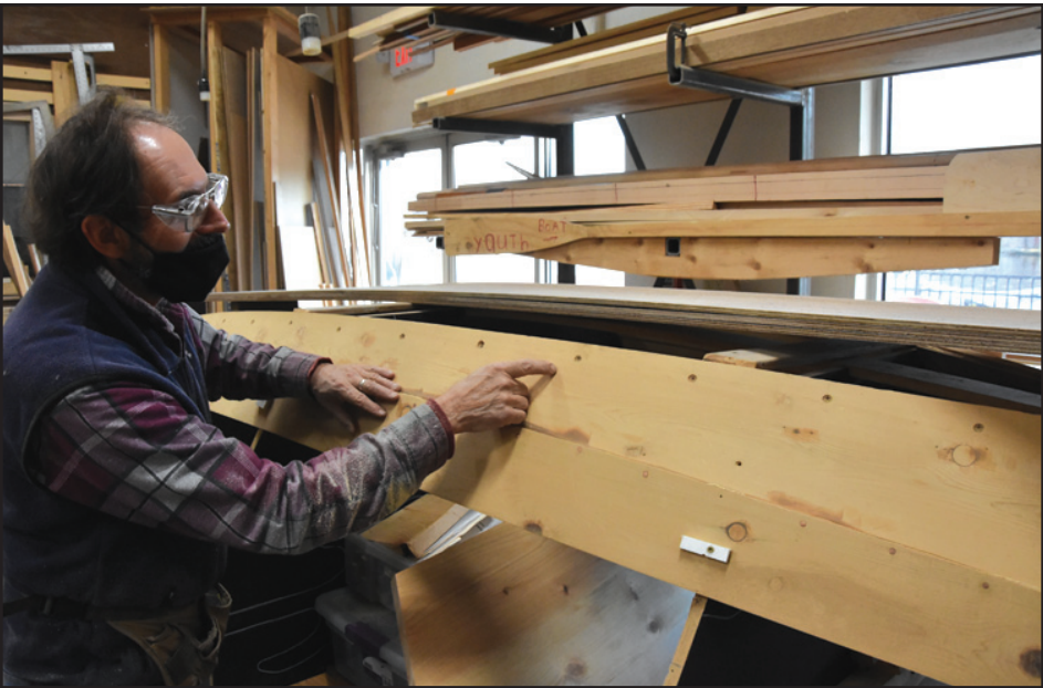
Chief Shipwright of the Wooden Boat School, Wayne Ford, verifying the location of the inner attachment point for the first strake (side board of the hull) and measuring to fit the next one as the project begins to move forward again. Photo by Jim Donick
