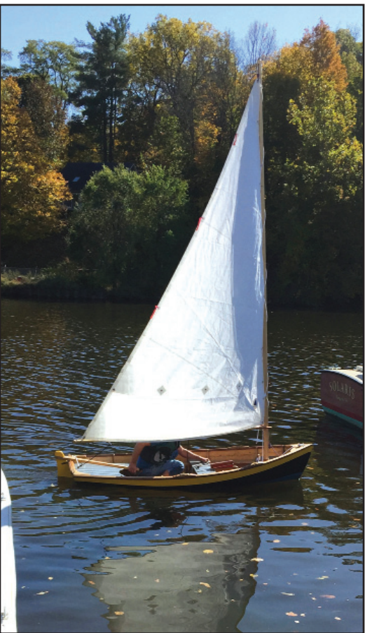
One of the projects of the last complete YouthBoat program class was to build a 10-foot long sailing dinghy, an Atkin "Nymph." The class built the boat, as well as all of the additional parts, the rudder, a dagger board (center board), and even the mast and boom. Here it is seen taking its maiden sail on the Rondout behind the Wooden Boat School. Courtesy photo
